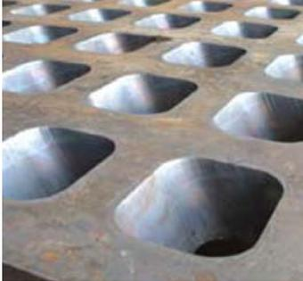
↳ Steel specialists Abraservice UK, one of Europe’s largest specialist steel processors and stockholders of abrasion resistant and high yield steel, have shown the Foundry industry how the use of CREUSABRO 4800 wear resistant steel for shake out screens can be extremely cost effective.
