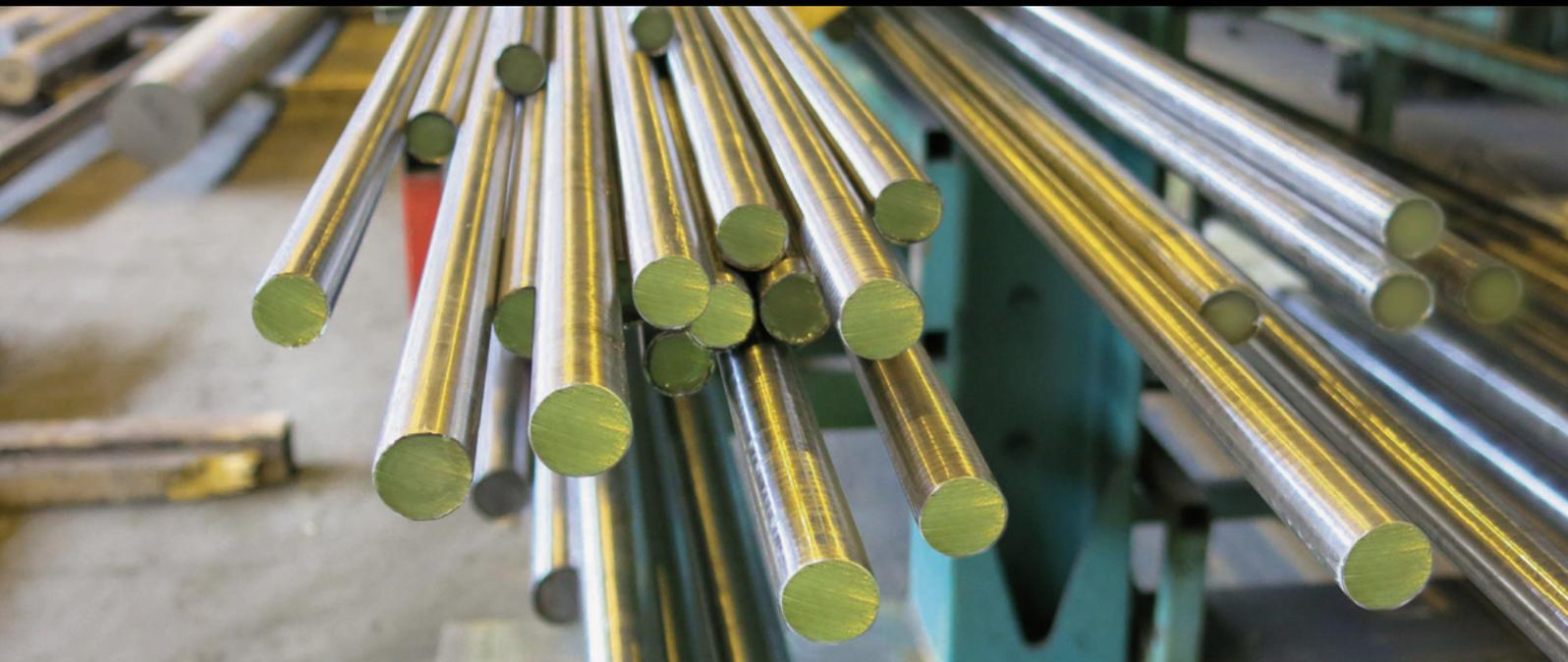
Toolox® in round bars, delivered heat treated to high tensile strength levels of typically 210 ksi, represents entirely new possibilities for product design. The need for heat treatments on standard steel grades is eliminated and the time-to-market becomes shorter.
