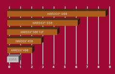
\*The calculations are based on sliding wear with granite.
