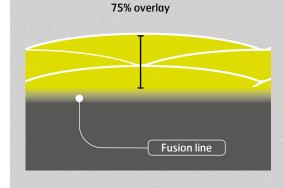
Duroxite® overlay plates and pipes are delivered with an overlay thickness guaranteed within  $\pm 10\%$ . This is consistent throughout the material and between individual plates and pipes.
