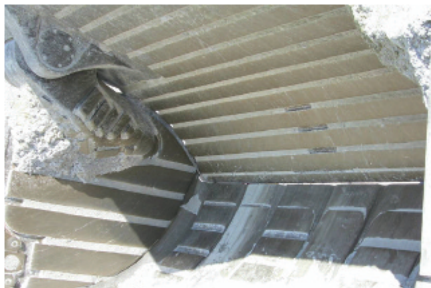
Minimal wear has occurred during the test programme retaining the integrity of the bucket operation. Small grooving in the structural base of the bucket can be seen
