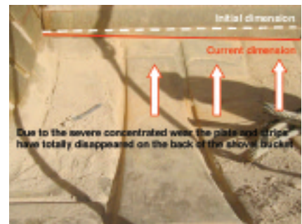
View showing the serious wear effect in the centre of the shovel bucket. Measurements were not possible on the plate and strips due to the severity of the wear
