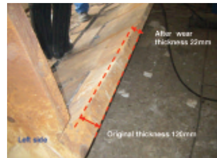
Measuring the wear effect from left to right on the back of the shovel bucket
