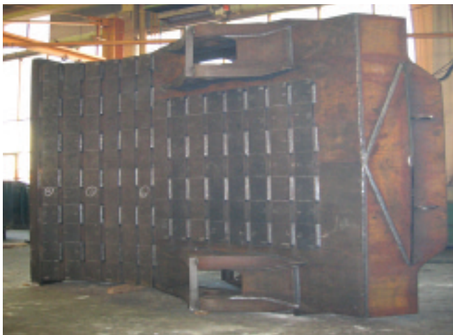
Beam on the back static part of the test bucket manufactured from a high-yield-strength steel, 120mm in thickness
