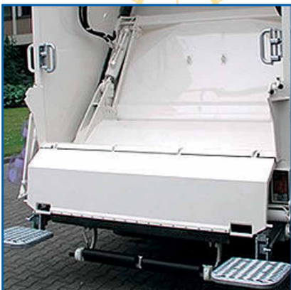
Refuse truck construction incorporating specialist wear resistant steel Creusabro 4800
